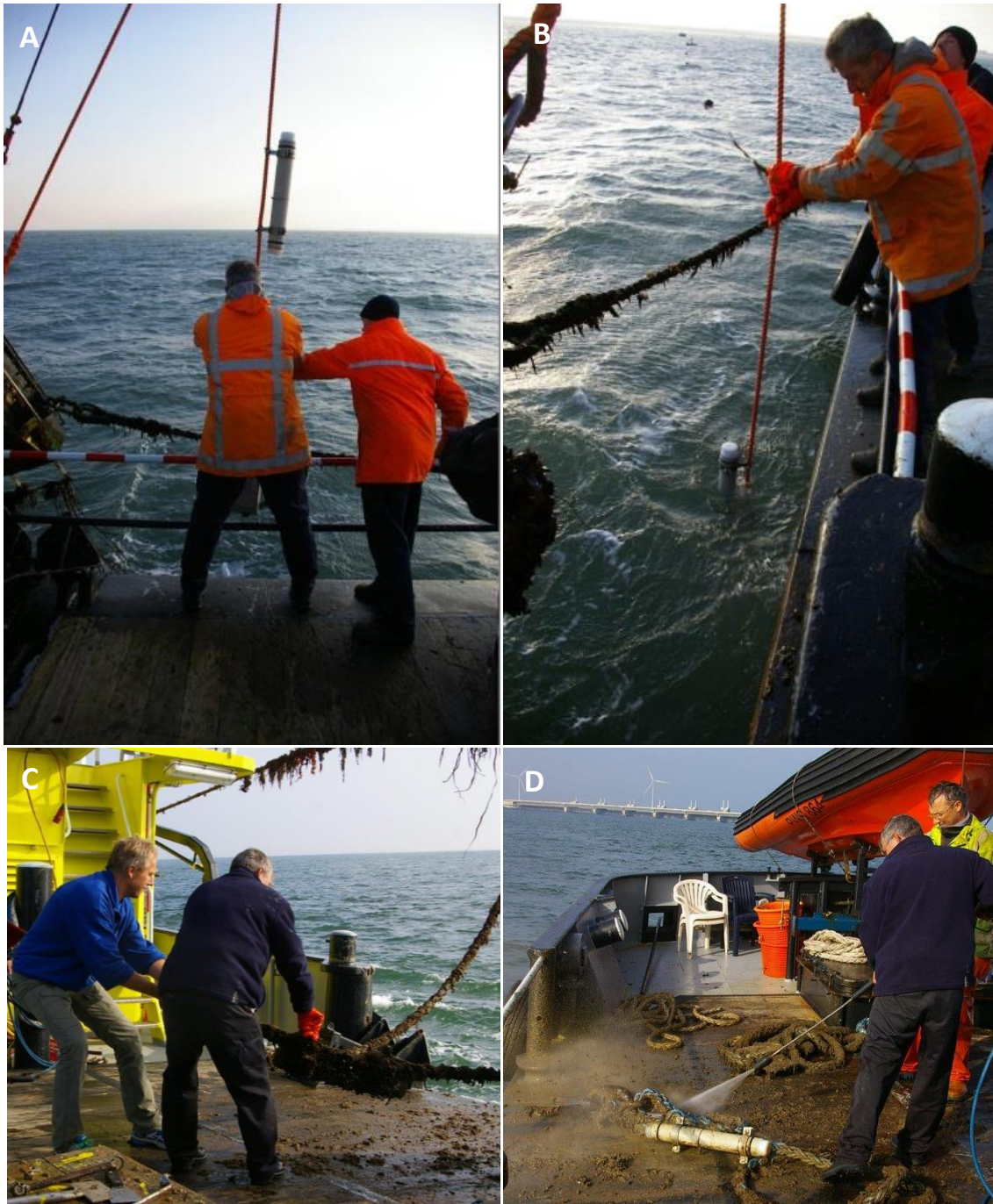
Figure 2 Handling of C-PODs. A: deploying the C-POD. B: attaching the C-POD to the safety line and deploying it into the water. C: retrieving the C-POD. D: Hosing and cleaning the C-POD after retrieval.
