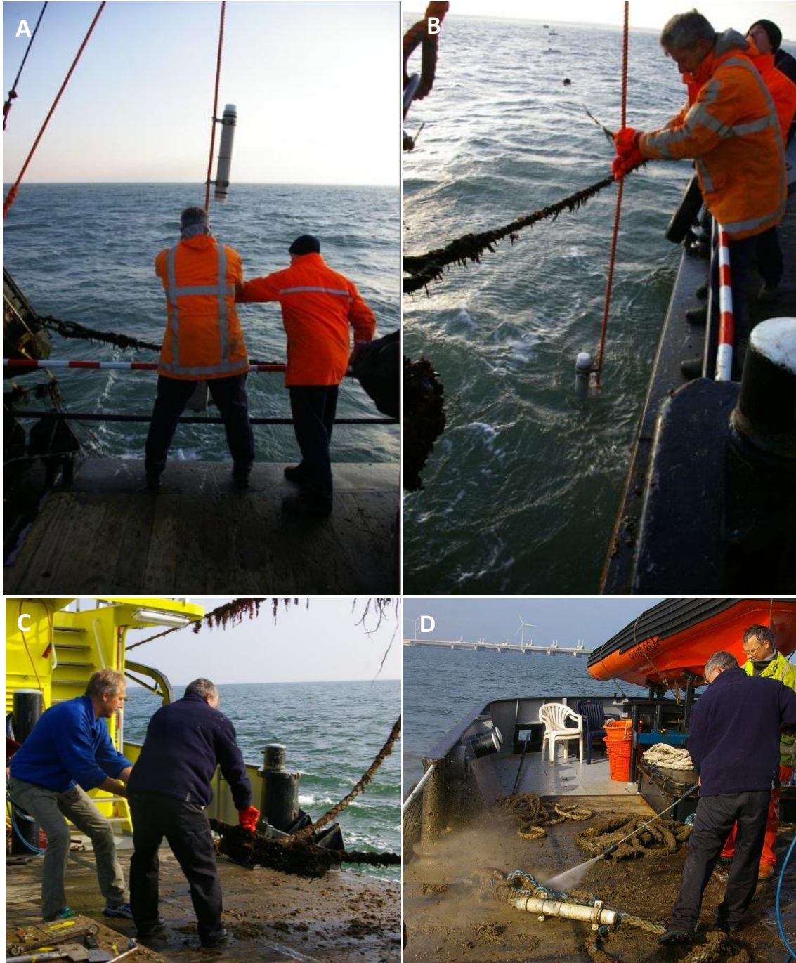
Figure 3 Handling of C-PODs. A: deploying the C-POD. B: attaching the C-POD to the safety line and deploying it into the water. C: retrieving the C-POD. D: Hosing and cleaning the C-POD after retrieval.
